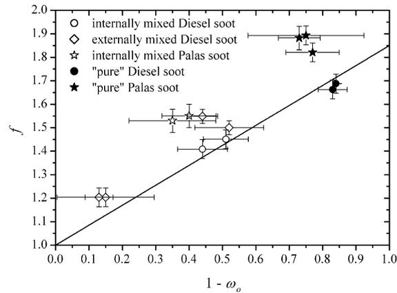
Fig. 4. Determined  $f$  values (a measure for the shadowing effect) at  $\lambda = 660$  nm vs.  $1 - \omega_0$  ( $\omega_0$  is the single scattering albedo for the particles in the airborne state). Different symbols are used to distinguish between different aerosols. The line is a fitted curve (Eq. (10)) which visualizes the trend for “pure” and internally mixed diesel particles and can be used for a correction of the shadowing effect.
