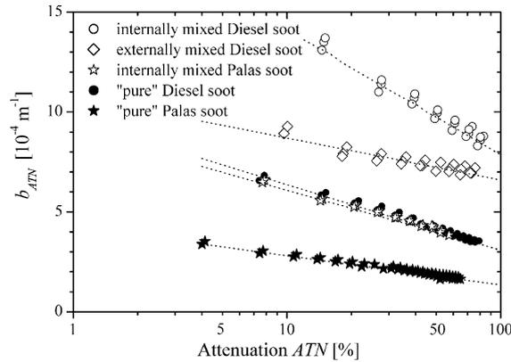
Fig. 3. Measured AE10 aethalometer signals (symbols) as a function of ATN for different aerosols. An empirical curve (dotted lines) was fitted to the data (Eq. (8), see text) which allows a parameterization of the observed shadowing effect.
