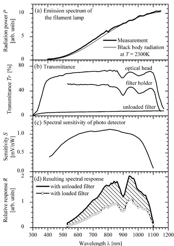
Fig. 1. Measured radiation power  $P$  of the filament bulb (a) and the transmittance  $T_r$  of the optical components of the AE10 aethalometer (b). Together with the spectral sensitivity  $S$  of the photo detector (c) the spectral response  $R$  (d) of this instrument was calculated with an unloaded and particle loaded filter (see text).
